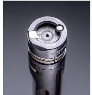
Each bolt face has a blade extractor and coil-spring-powered, plunger-style ejector. The opposing position ensures reliable cycling.
