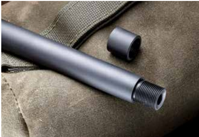
The match-grade, cold extruded barrel measured 22 inches, having a 1-in-8-inch twist rate. The end of the barrel is threaded M14x1, but an included adapter changes that to the common 7/8x24.
