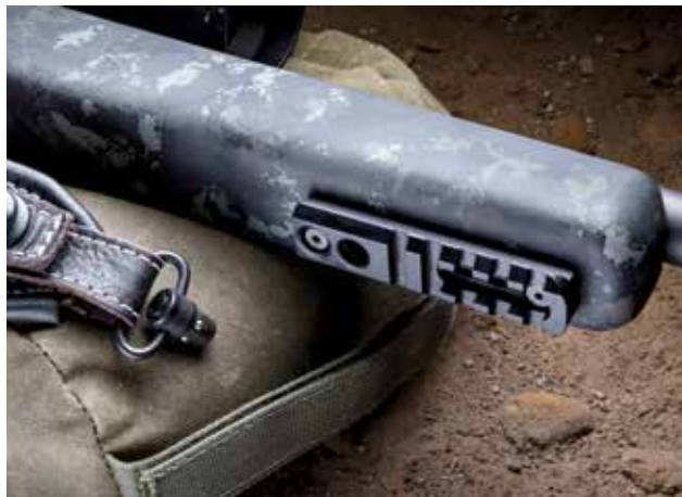
A length of accessory rail is installed at the front of the handguard. A sling swivel stud can be found at the rear, just under the recoil pad.
