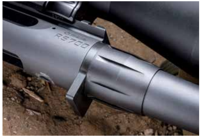
The recoil lug sits between the barrel and action, which are connected by a 1 1/16x16 UN thread pitch. This thread pitch offers potential for aftermarket barrel changes in the U.S.
