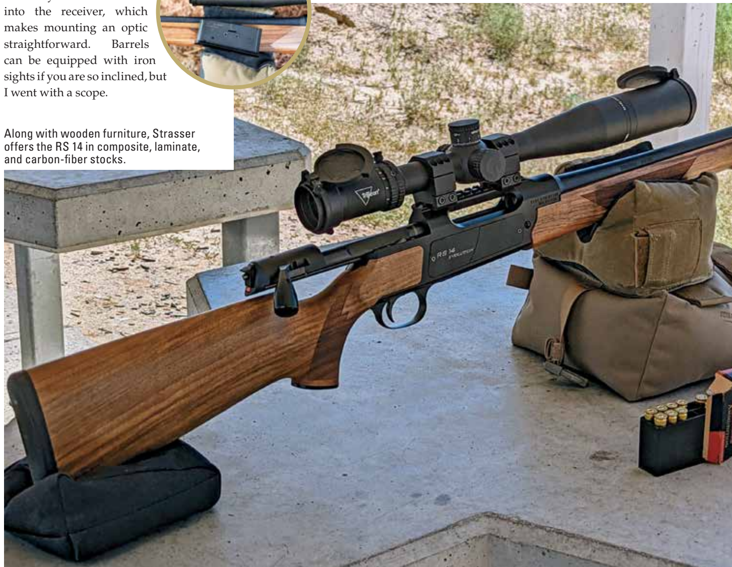
The RS 14 is a switch-barrel design that facilitates a number of different cartridges.
