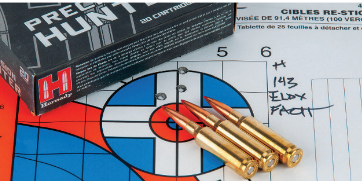
Best accuracy was obtained with Hornady's 6.5 Creedmoor 143-grain ELD-X Precision Hunter ammunition. Average group size was just under one MOA.
