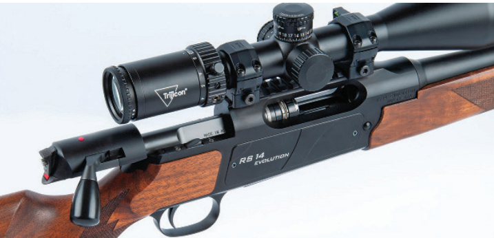
A Picatinny rail is machined integral with the top of the action and makes mounting a scope easy. Because of the design of the rear of the action, a right-handed bolt assembly can be switched for a left-handed version with no fitting or tuning required.
