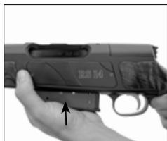
4.9 Insert magazine into magazine well until it snaps into place.
