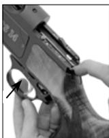
4.7 Now put the trigger assembly back into the receiver.
