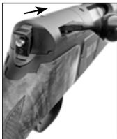
4.8 Now insert the bolt into the receiver. For this the bolt handle must be in the rearward position and the locking elements of the bolt-head must be in the retracted state (not expanded). Otherwise it is not possible to insert the bolt. Pay attention to an exact positioning of the bolt i.e. horizontal to the receiver to align the bolt with the guide.
